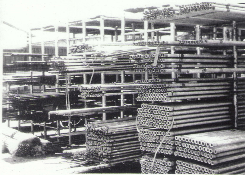
19 Trestles provide a suitable means of storing pipes and tubes © D A Jessop 20 Lighter tubes can be placed in a simple rack © D A Jessop
