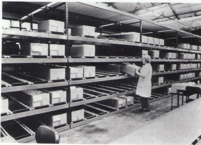
8 Cage pallets being handled by a sideloading reach truck (By courtesy of Materials Handling Equipment (GB) Ltd.) 9 A live storage installation. The boxes are fed to the operator by gravity (By courtesy of Stembeck Ltd.)
