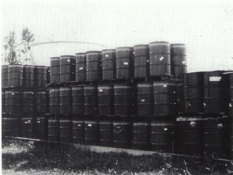
4 (above) Unit loads stored in pallet racking (By courtesy of Link 51 Ltd.) 5 (below) Four oil drums strapped to a pallet make a stackable unit load © D A Jessop
