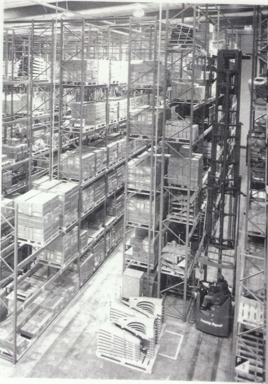
11 High rise narrow aisle pallet racking (By courtesy of Lansing Ltd.)
